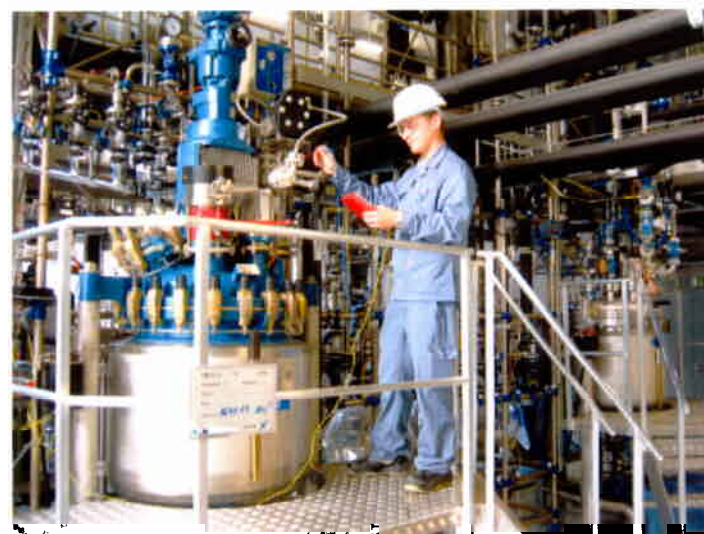
Fig. 3. Shift worker operating a typical 160L SSP reactor
